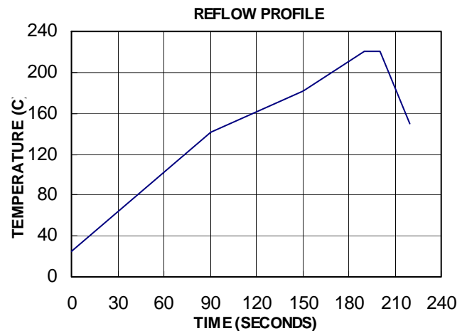
Figure 18 SMT Reflow Profile
